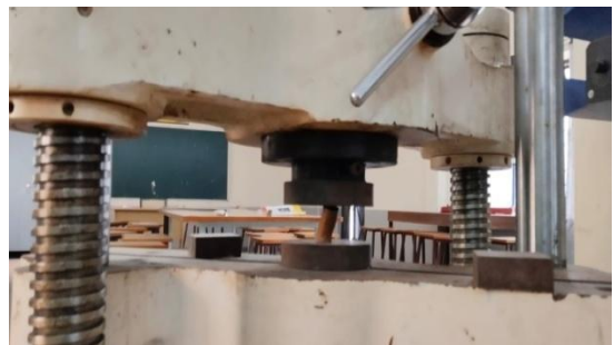
Fig 11. Al-6061 & Copper placed on UTM
