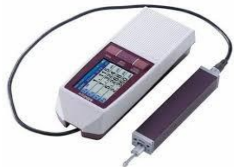
Fig 1. Profilometer surface roughness tester.
