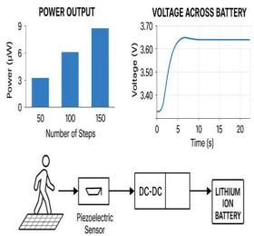
This proportional rise confirms that the piezoelectric plates effectively convert mechanical stress into electrical energy and that the system performs more efficiently when subjected to higher footfall.
